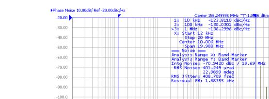
Example A1: 156.25MHz LVDS clock, generated by VersaClock 6 with a 25MHz crystal
