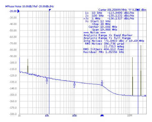
Example B1: 156.25MHz for FPGA and 100MHz for PCI Express®
