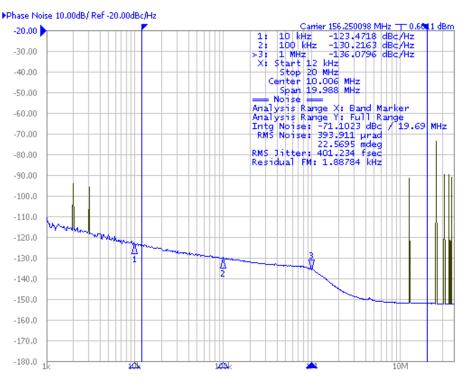
Example B2: 156.25MHz for FPGA, 2 X 100MHz for PCI Express and 125MHz for Giga Bit Ethernet
