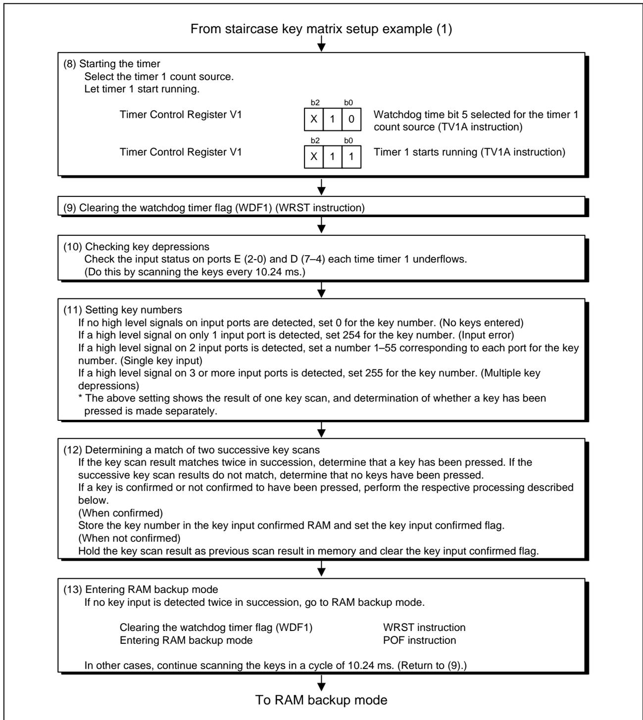
Figure 4.4 Staircase Key Matrix Setup Example (2)
