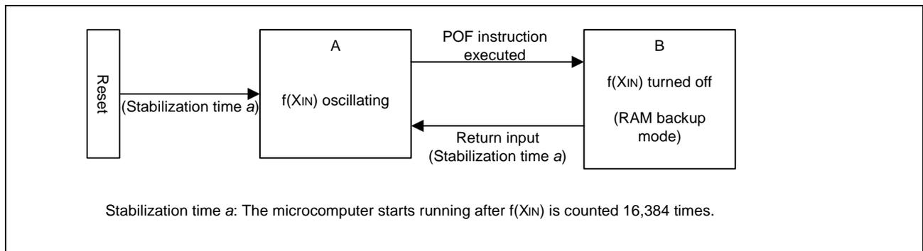
Figure 4.1 State Transition Diagram
