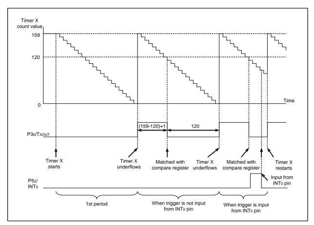
Figure 3.2 TXOUT Output Waveform
