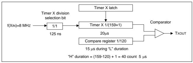
Figure 3.1 Timer Connection and Setting of Division Ratio
