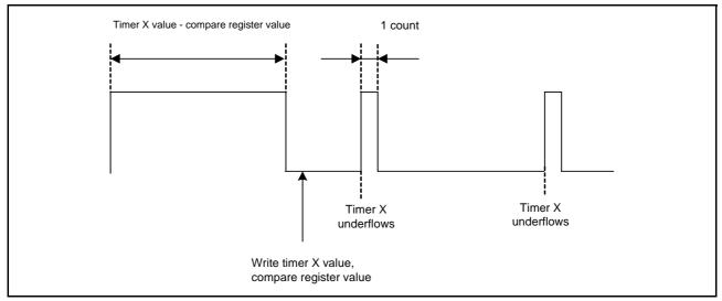
Figure 4.2 Example of IGBT Control Signal Output when Same Value is Set to Timer X and Compare Register
