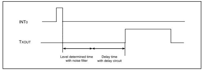
Figure 4.3 Example of IGBT Control Signal Output of TXOUT Pin by Trigger Input to INTO Pin
