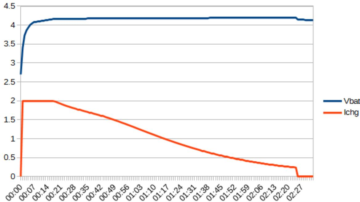
**Figure 11. Measured Charging profile plot**
