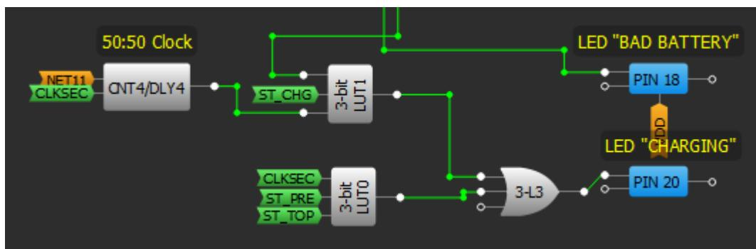
**Figure 7. Charging indicator circuit**
