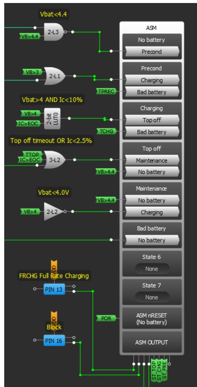
Figure 4. ASM Connections
