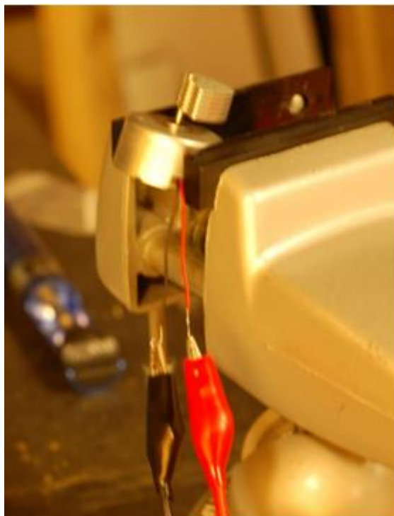
Figure 11: Vibration motor in a vise
