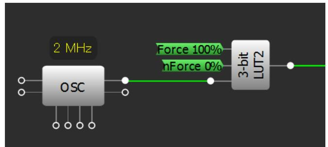
Figure 9. Clock control when PWM duty is 0 or 100%
