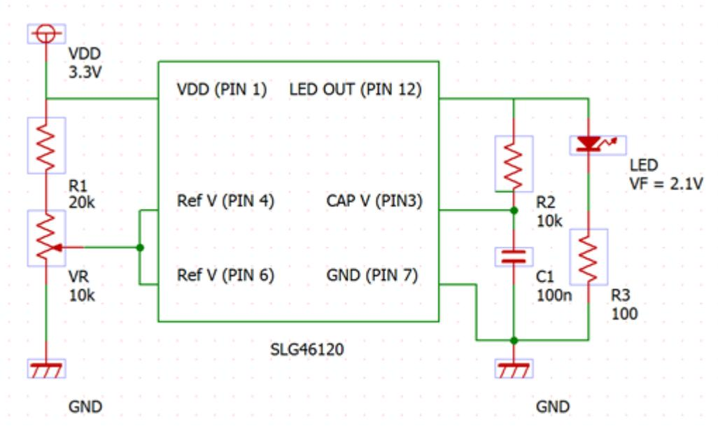
Figure 1. External Circuit
