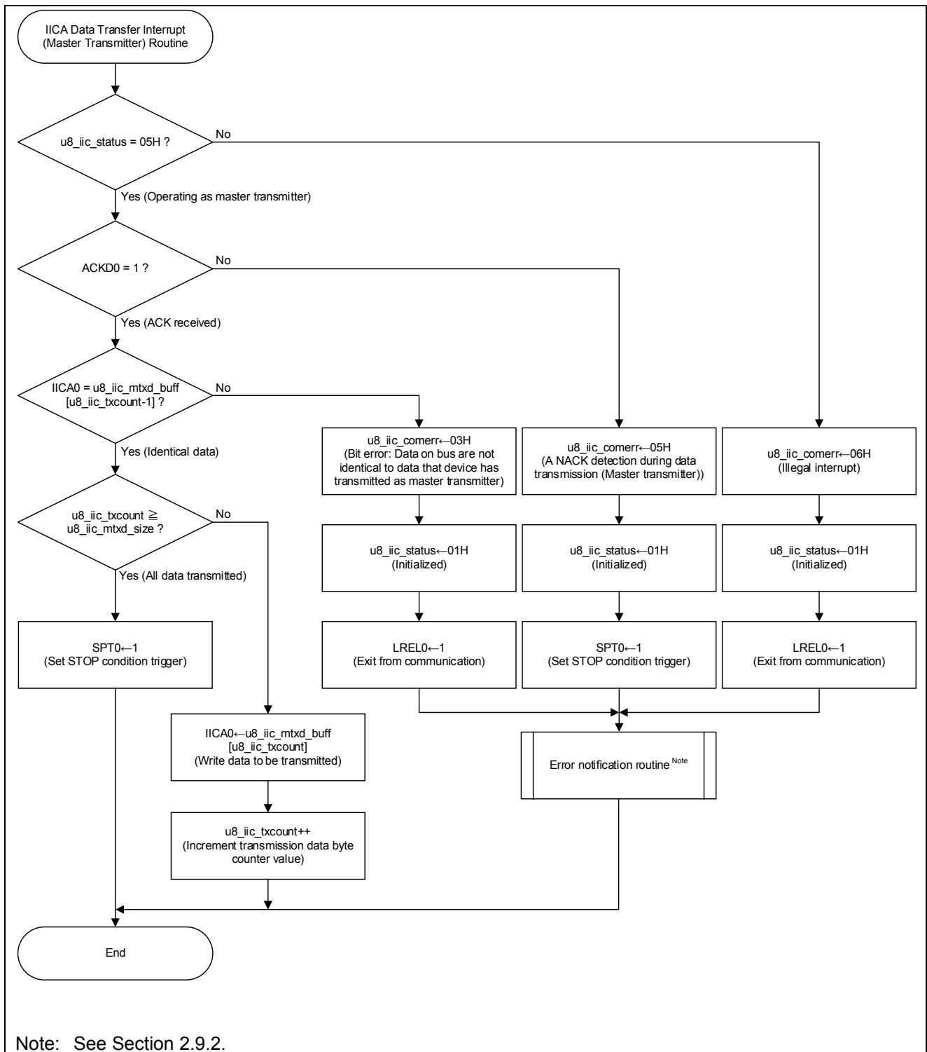
Figure 2-19. IICA Data Transfer Interrupt (Master Transmitter) Routine
