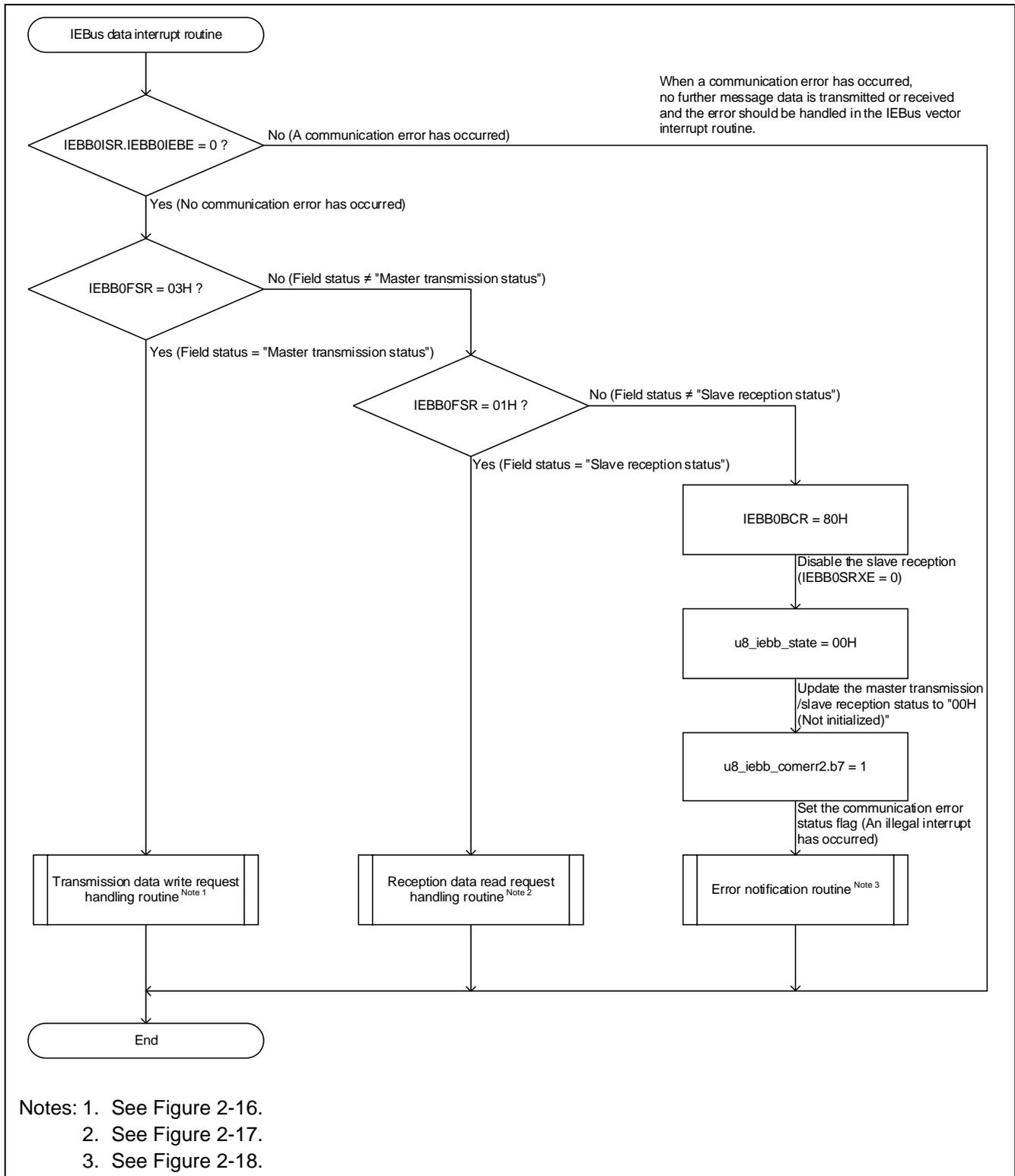
Figure 2-15 IEBus Data Interrupt Routine
