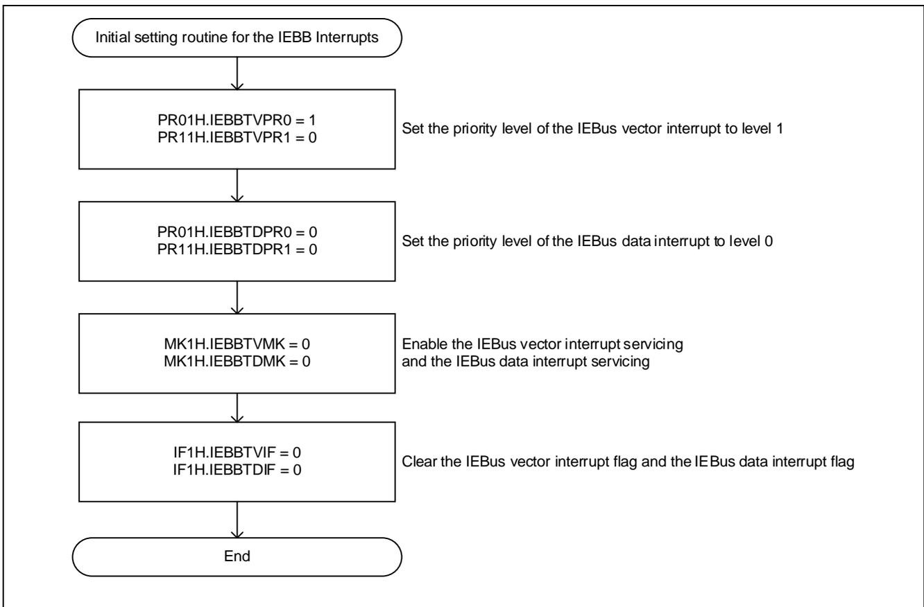
Figure 2-6 Initial Setting Routine for IEBB interrupts
