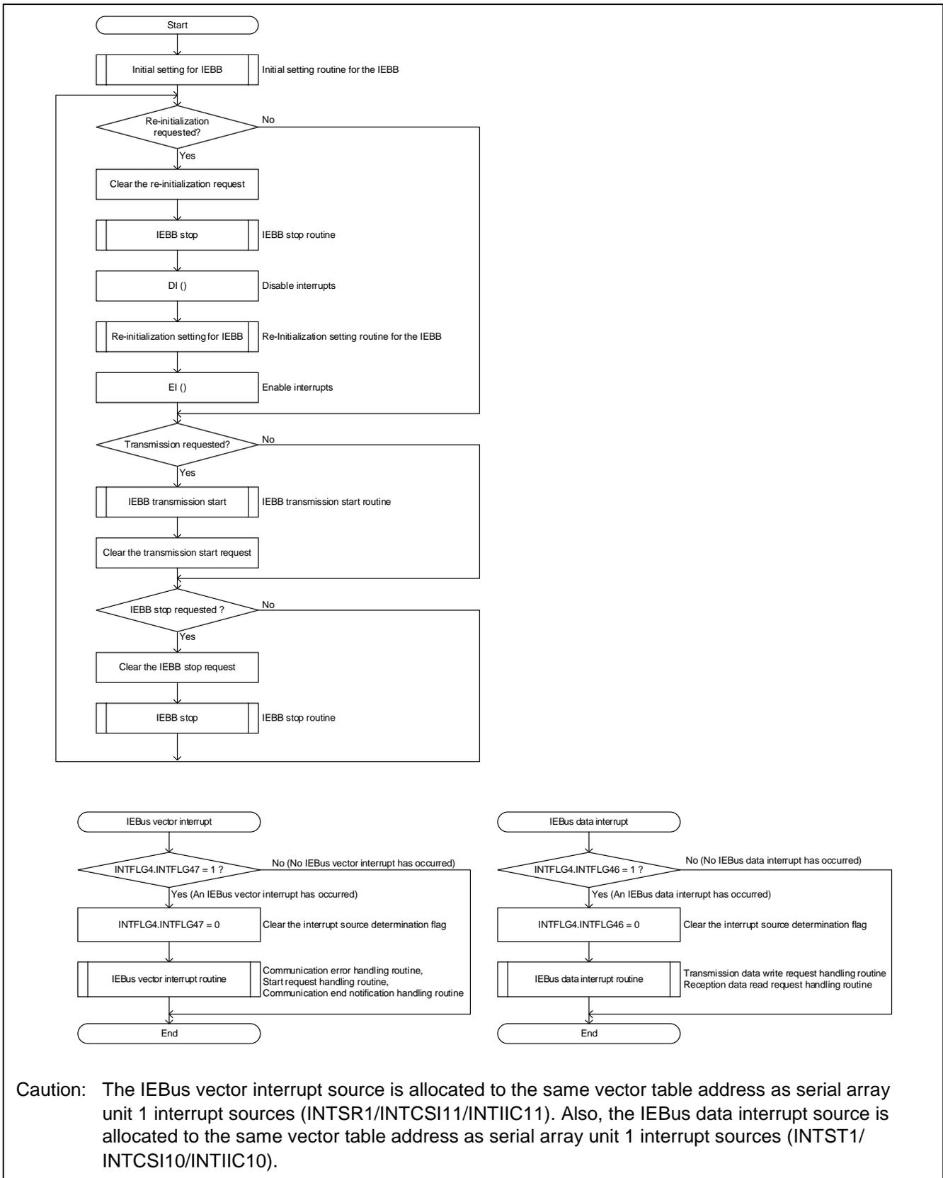
**Caution:** The IEBus vector interrupt source is allocated to the same vector table address as serial array unit 1 interrupt sources (INTSR1/INTCSI11/INTIIC11). Also, the IEBus data interrupt source is allocated to the same vector table address as serial array unit 1 interrupt sources (INTST1/INTCSI10/INTIIC10).
