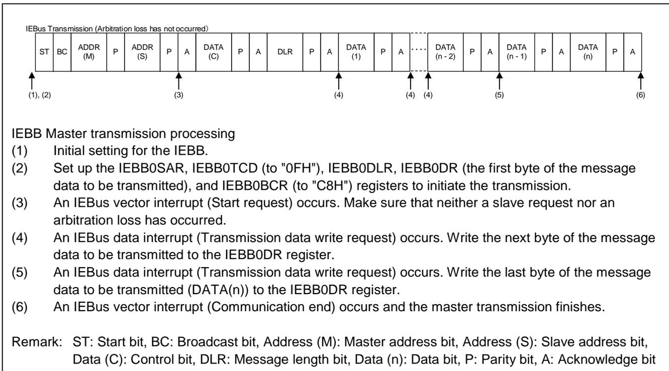
Figure 2-2 Master Transmission Processing (Timing Chart)
