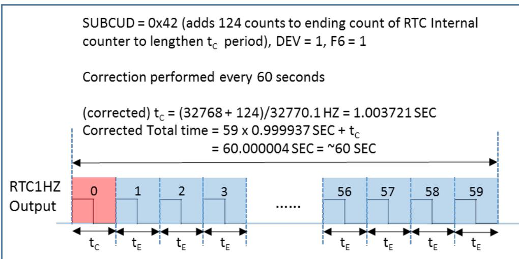
**Conclusion:** For a smaller error range of +/-63 PPM, the “fine” setting of 1.02 ppm steps can be used. In this mode, Watch error correction can be used to get accurate 60 second intervals over the long term. Using the finer Watch error correction steps of 1.02 PPM allows closer correction to 0 ppm elapsed time error, but there can be up to 1.02 PPM quantization error, even if the initial PPM delivered error and temperature drift errors are offset and applied perfectly.
