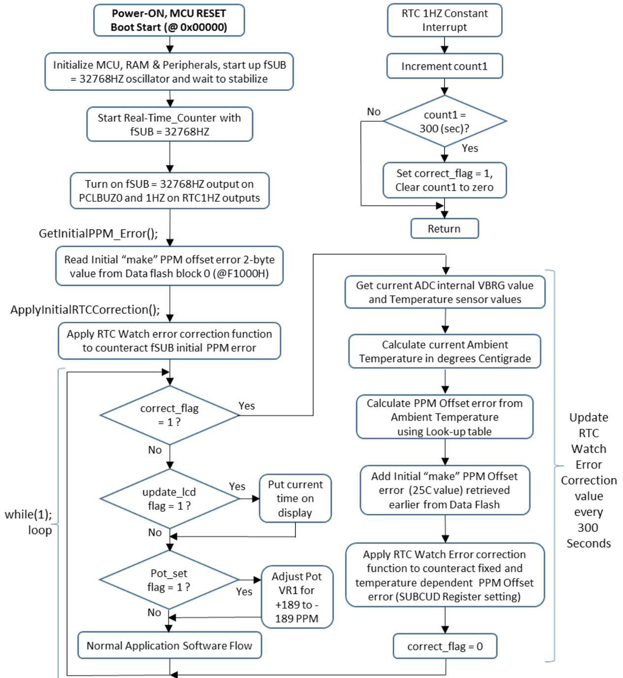
When the resulting PPM error is in +64 to +189 PPM or -64 to -189 PPM range, then SUBCUD register is set for the RTC Watch correction automatically performed once every 20 second counts (SUBCUD DEV bit = 0) and is applied in 3.05 PPM steps. When the resulting PPM error is in -63 to +63 PPM range, then SUBCUD register can be set for the RTC Watch correction automatically performed once every 60 second counts (SUBCUD DEV bit = 1) and is applied in 1.02 PPM steps.
