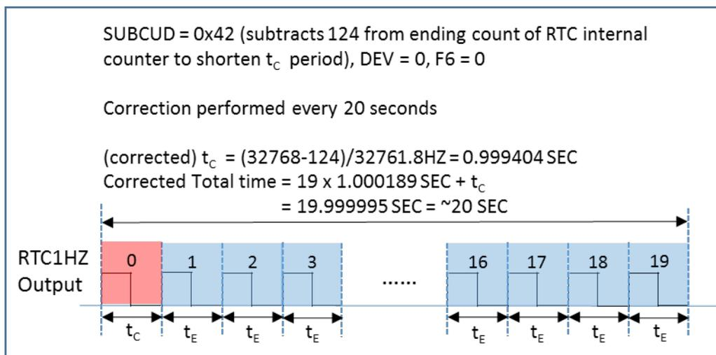
**Conclusion:** For a large error of -189 PPM the coarse setting of 3.05 PPM correction steps must be used. Watch error correction can be used to get accurate 20 second intervals over the long term. Since the Watch error correction can only
