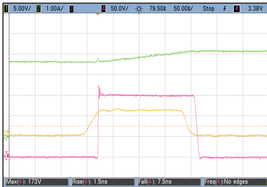
Figure 3 – Waveforms for 150V_{IN} to 5V_{OUT} @ 4A ( 200kHz ) Buck Convertor.
