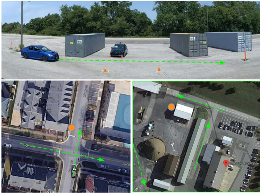
Fig. 2 Initial data was collected on compact sedan ego vehicles (e.g. Toyota Corolla.) The system was tested in a variety of actual neighborhoods, complex obstacle areas and purpose-built closed courses.
