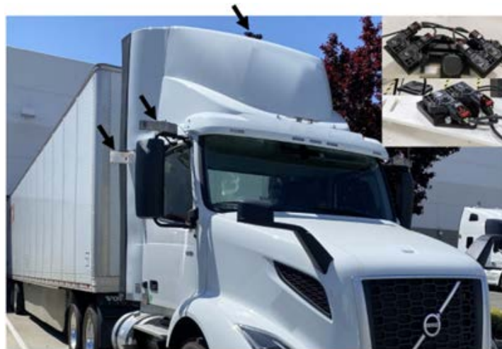
Fig. 3 We are also working with an autonomous trucking company to instrument heavy vehicles in live tests ranging from engine idling to highway speeds. Arrows show test array locations. Inserts (top right) show exterior automotive rated microphone modules arrays which can be integrated behind bodywork or fairings in production.
