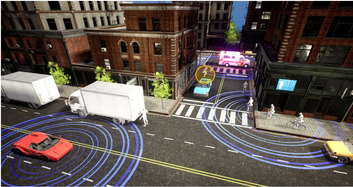
Fig. 1 Typical use case is nearby targets in slow speed, obstructed view situations. Sirens will be detected at greater range under wider driving conditions. Image is copyright © Renesas Electronics, used with permission.
