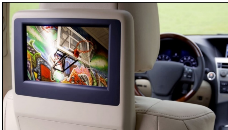
Figure 6: The TW8844/45 can simultaneously drive two rear seat video displays with different content
