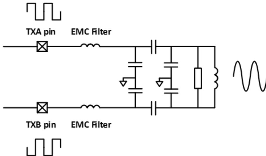
Fig. 2: the conventional architecture of NFC controllers used in today's contactless payment terminals. (Image credit: Panthronics)
