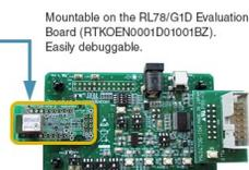
Mountable on the RL78/G1D Evaluation Board (RTK0EN0001D01001BZ).
