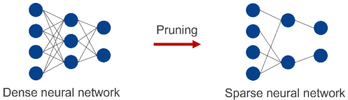
Figure 7: Reduction of Model Weight by Pruning
