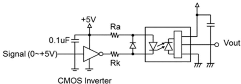
**Figure 4.** Divided resistor input to improve CMR
