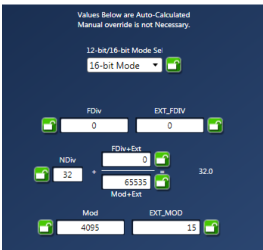
Figure 3. 8V97053 Feedback Divider Settings for 1.6 GHz Output using a 100 MHz PFD Frequency
