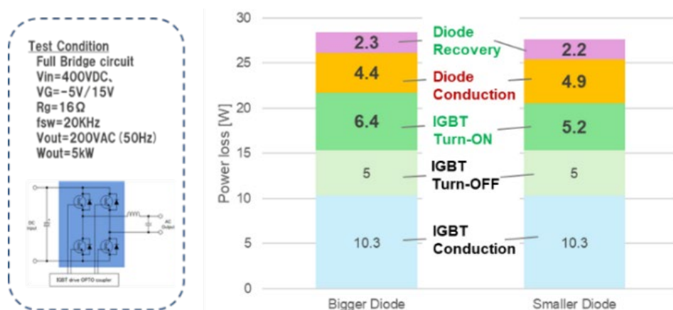
Figure 5 Total power loss simulation conditions and results
