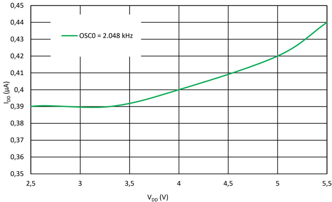
Figure 4. SLG47105 OSC0 Current Consumption vs. V<sub>DD</sub>
