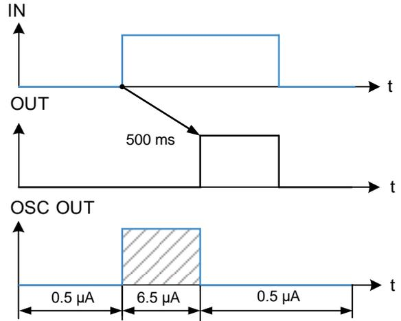
Figure 5. Example of Auto Power-On Function
