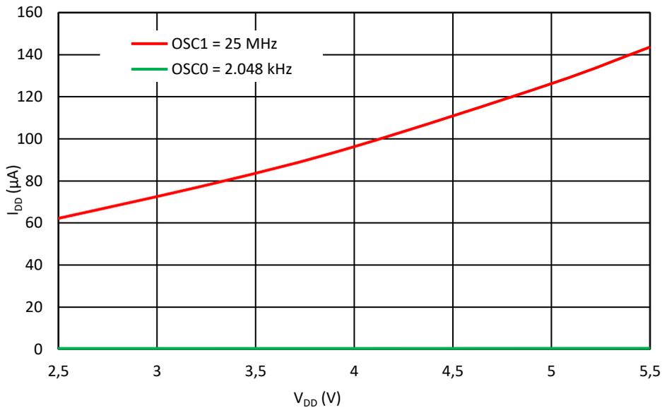
Figure 6. OSCs Current Consumption vs. VDD
