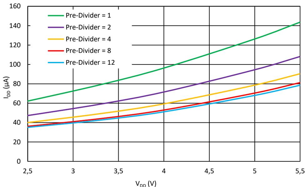
Figure 3. SLG47105 OSC1 Current Consumption vs. V<sub>DD</sub> for Different Pre-dividers
