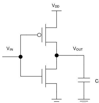
Figure 2. CMOS Inverter
