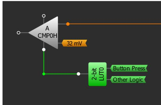
Figure 7. Power-Up Configuration Controlled by Logic
