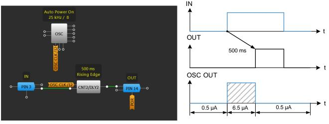
Figure 5. Example of Auto Power-On Function
