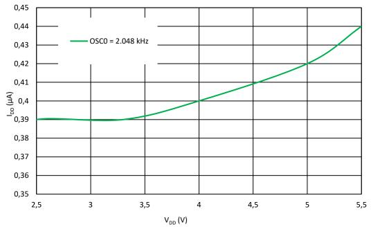
Figure 4. SLG47105 OSC0 Current Consumption vs. VDD
