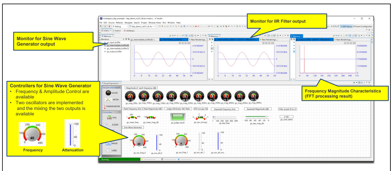
Figure 1 Sine wave generation processing console (e 2 studio)
