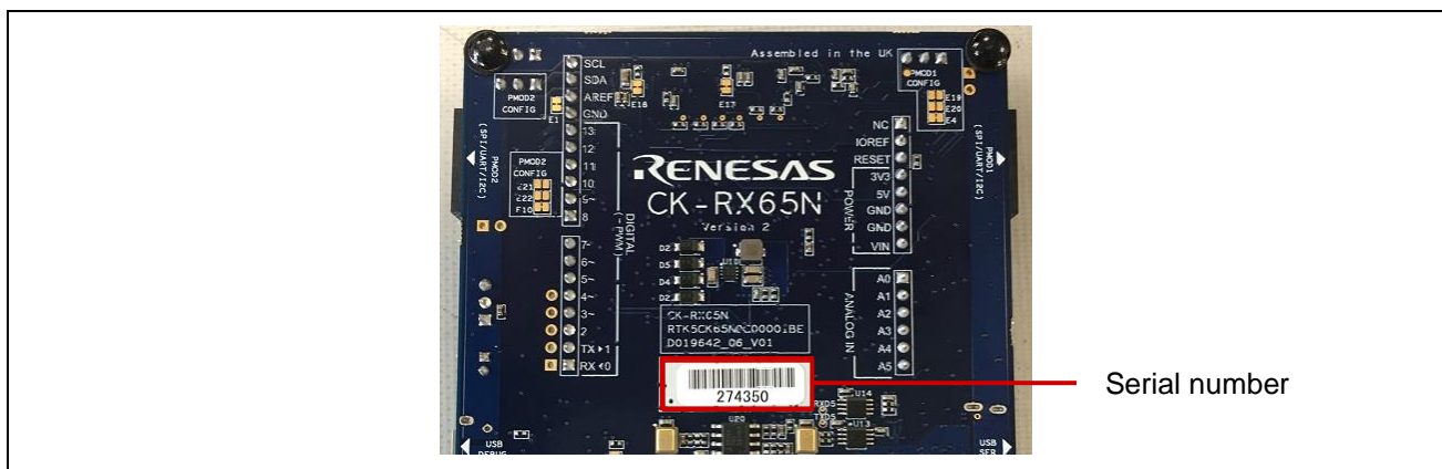
Figure 3 Location of the serial number (Bottom view of the CK-RX65N v2 board)
