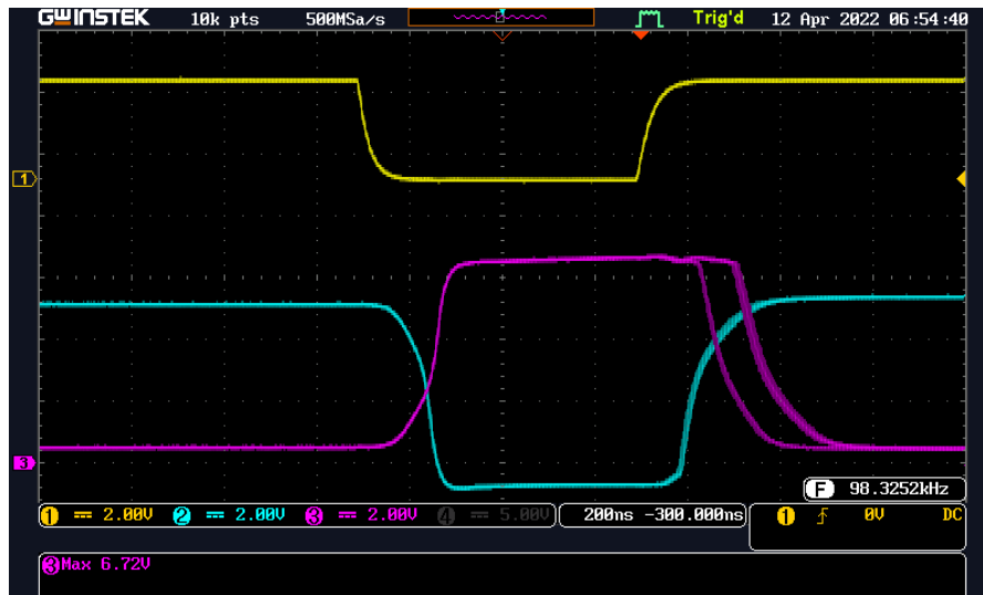
Figure 4 Shifted falling edge
