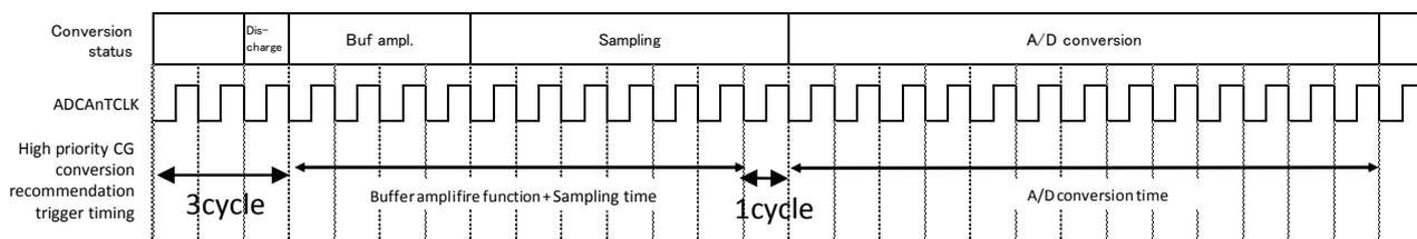
Example condition: Discharge function: ON, Buffer amplifier function: ON, ADCAnCTL1.ADCAnCTYP=0
