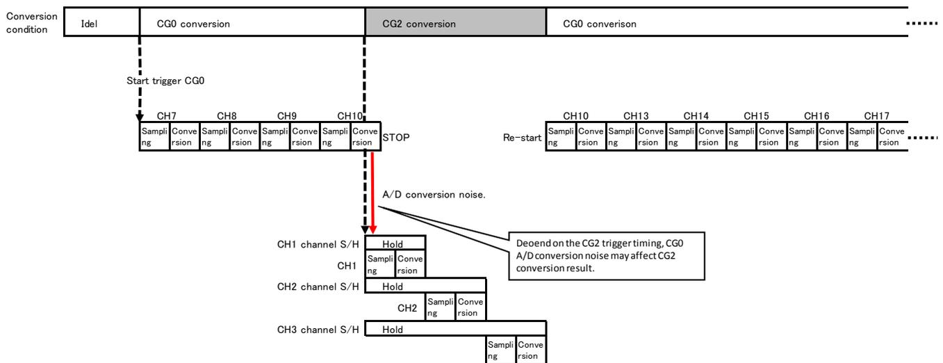
Note: The fluctuation of conversion error depends on the external circuit and devices mounted on the customer board.
