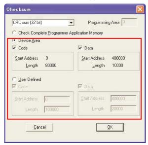
After clicking the OK button, the following information will be displayed in the File Checksum area of the programmer parameter window.
