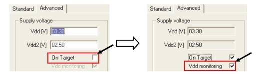
Caution When this function is disabled, the product can be used even if the VDD pin of the target system and that of the PG-FP4 are not connected, as long as the VDD generated in the target system and the VDD of the output signal generated by the PG-FP4 match.
