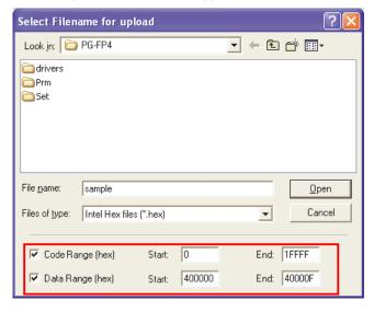
**Caution** Specify twice the required for the data range in order to accommodate the ID tag data. Example: When uploading 16 bytes of data flash data from address 400000, specify 32 bytes.
