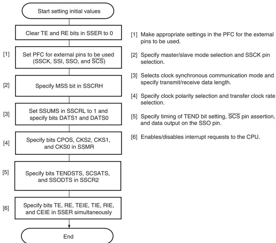
**Figure 14.12 Example of Initial Settings in Clock Synchronous Communication Mode**
