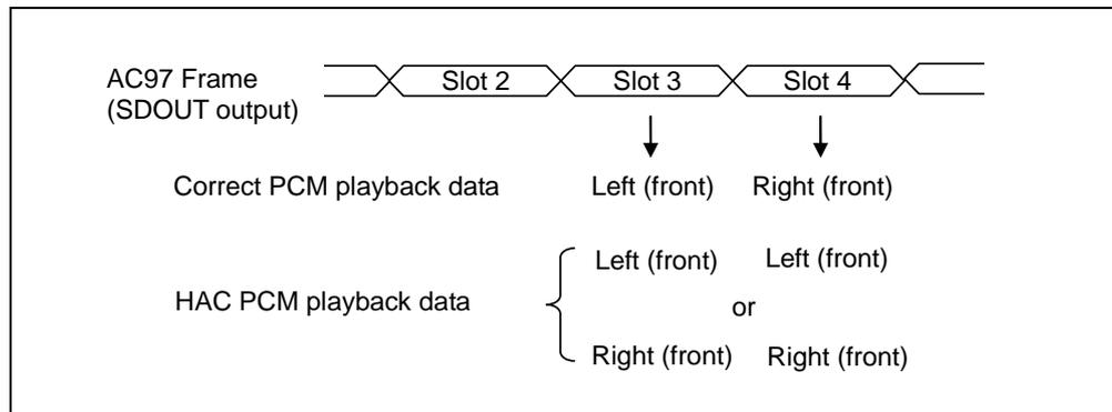
Figure. 20-Bit PCM Playback Data in TX DMA Enable
