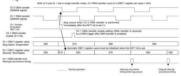
The following registers are buffer registers with a 2-stage FIFO configuration of master and slave. If these registers are overwritten during a DMA transfer or in the DMA-suspended status, the value is written to the master register, and reflected in the slave register when the DMA transfer of the overwritten channel is terminated.
