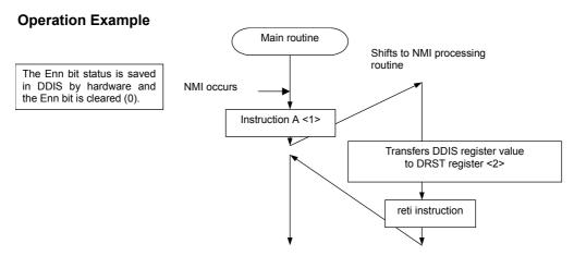
When the Enn bit of the DCHCn register is set to disable or enable DMA using instruction A, the disable/enable status of each DMA channel is inconsistent in <1> and <2>. As a result, the normally suspended DMA transfer cannot be restored correctly.
