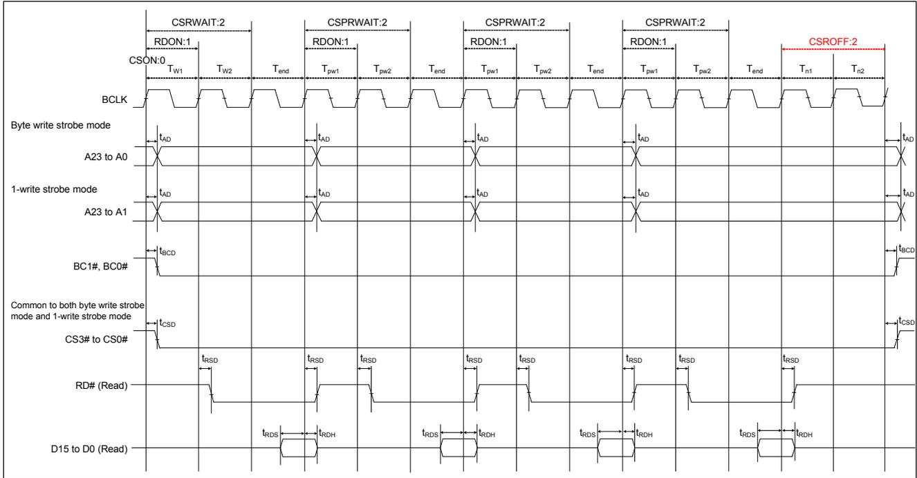
Description of CSWOFF in Figure 41.29 External Bus Timing/Page Write Cycle (Bus Clock Synchronized) is corrected as follows:
