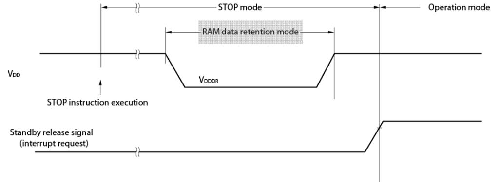
**10. 35.9 Data Memory STOP Mode Low Supply Voltage Data Retention Characteristics (Page 1294)**
