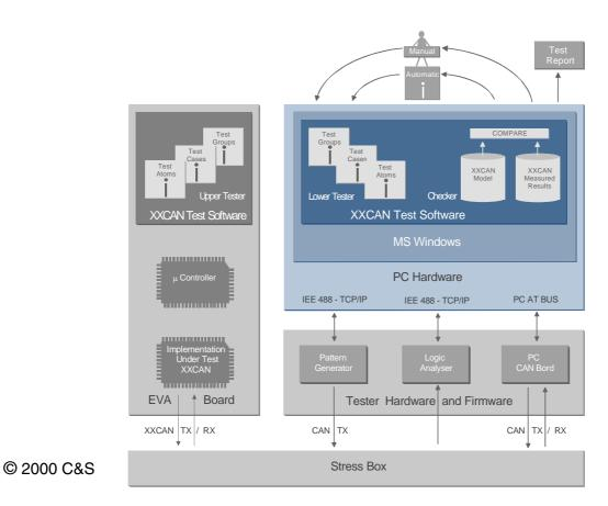
Figure 2-1 CAN Conformance Test System Overview
