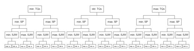
Figure 4-1 Bit Timing Test Cases
