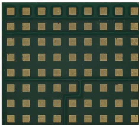
Figure 2. Typical Power Tower Bottom View - RRV29830
