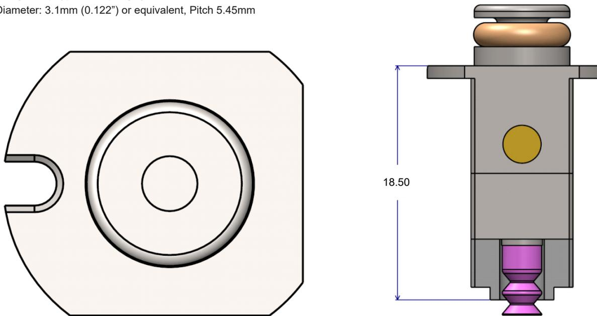
Figure 6. Suggested Power Tower Pickup Tool – Top and Side View
