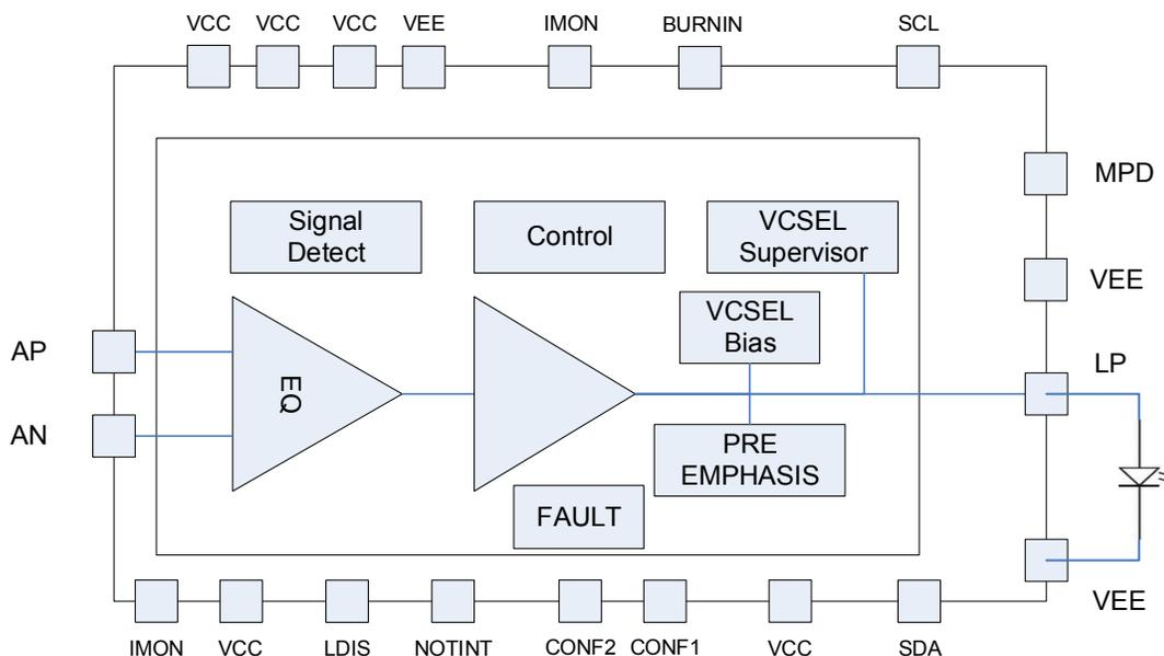
Figure 1: Device Diagram
