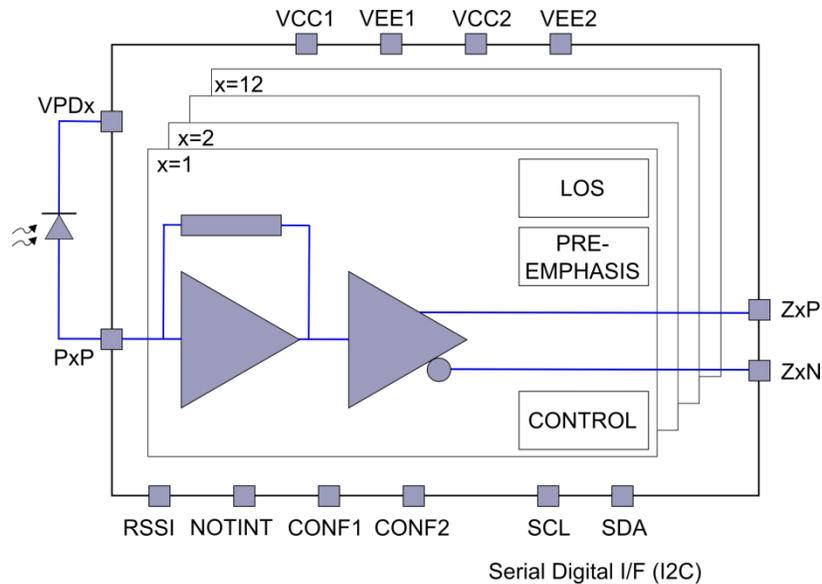
Figure 1. Block Diagram
