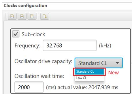
Figure 3-3 New selection of Standard CL in Sub-clock oscillator
