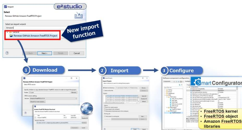
Figure 3-1 Configure Amazon FreeRTOS project using Smart Configurator in e<sup>2</sup> studio
