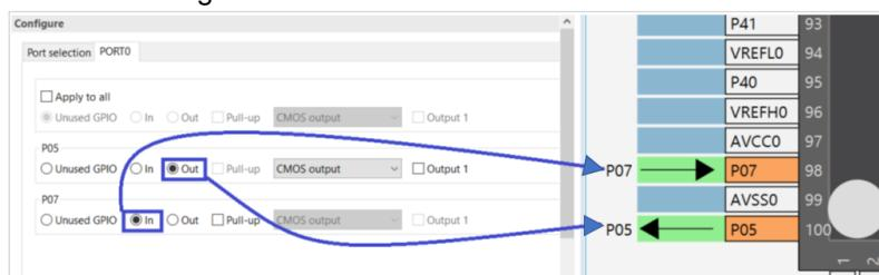
Figure 3-2 Ports direction on MCU Package view
