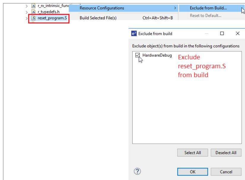
**Figure 5-2 Workaround of build error in CCRX project**
