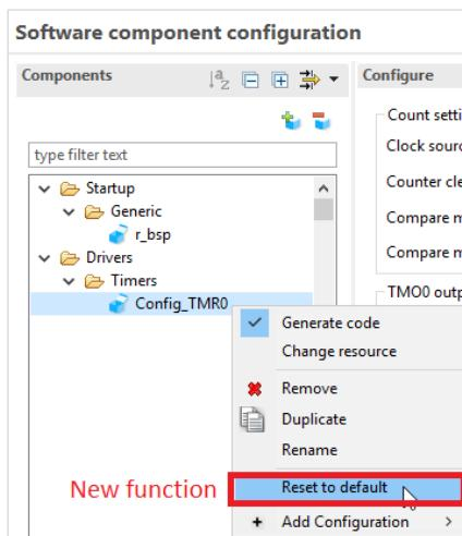
Figure 3-4 New function of Reset to default settings
