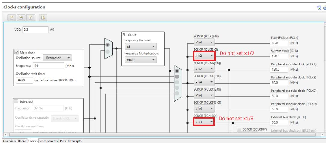
Figure 5-1 Limitation of clocks configuration in RX72M group devices
