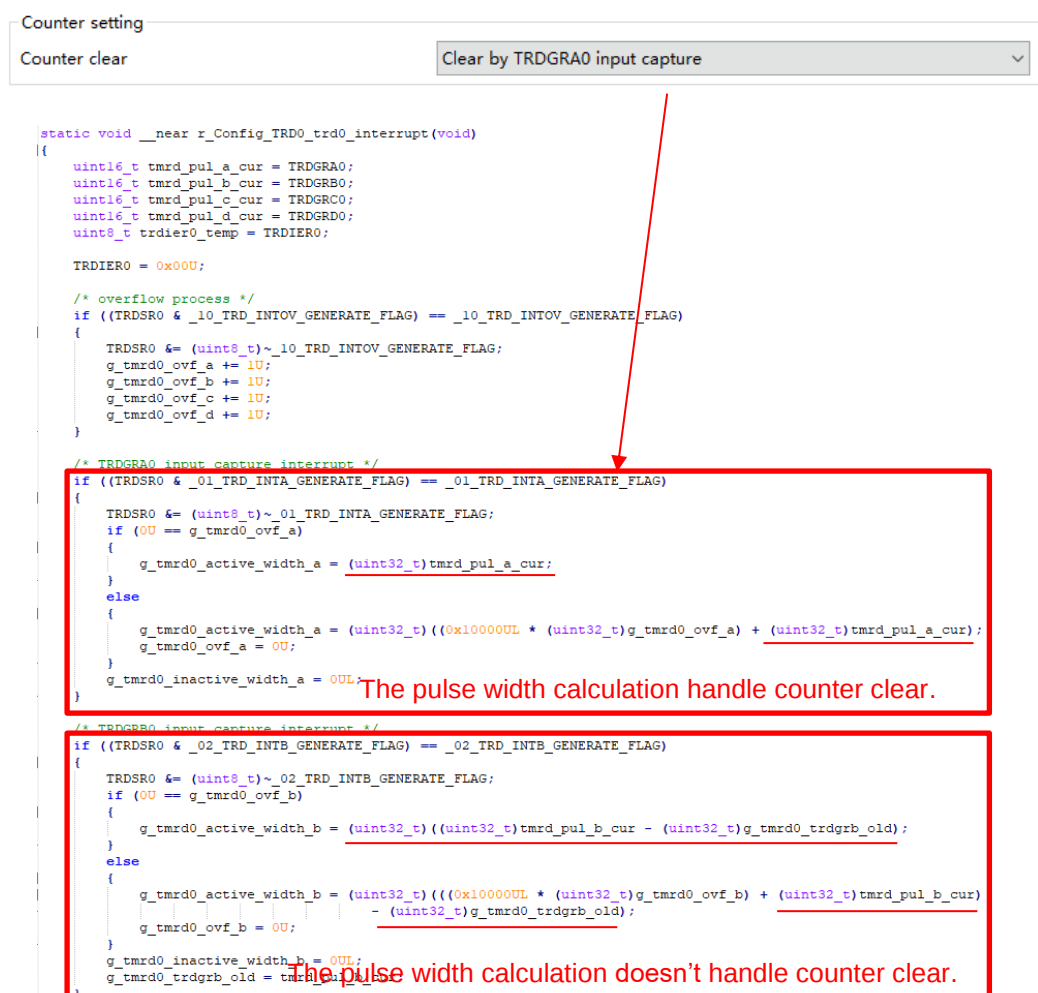
Figure 6-3 Counter clear setting in Input capture function
