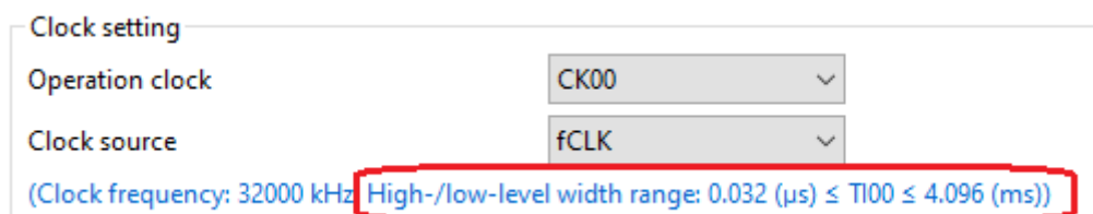
Figure 6-8 High/Low level width min value
