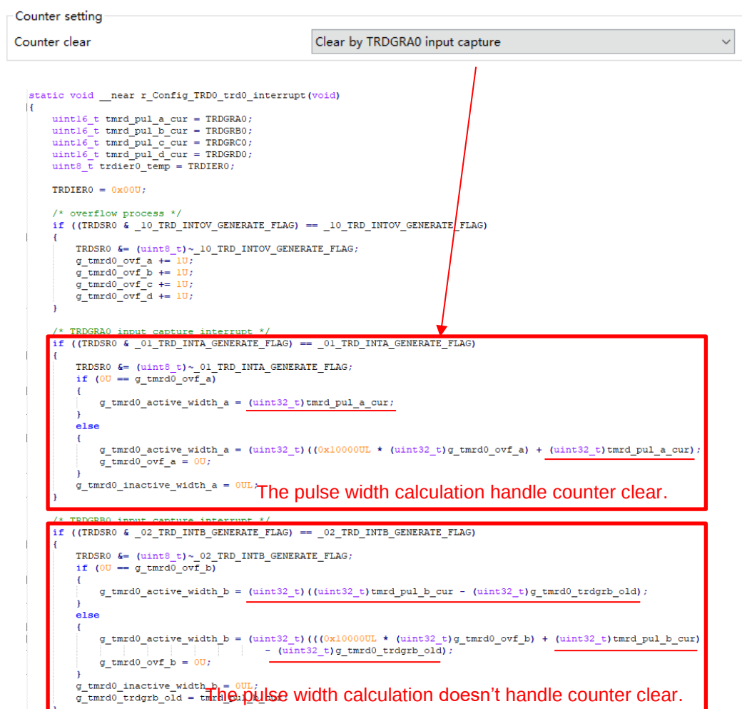
Figure 6-3 Counter clear setting in Input capture function
