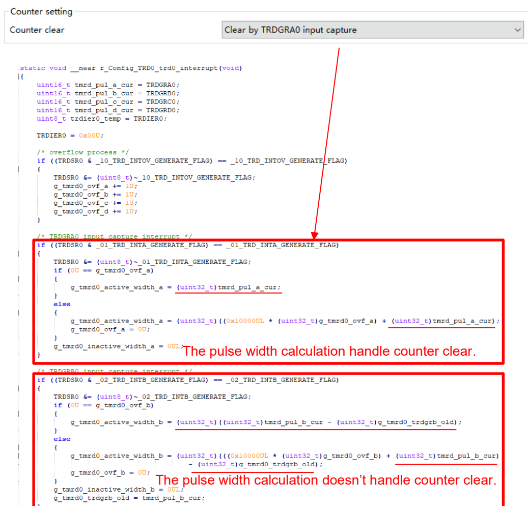
Figure 6-3 Counter clear setting in Input capture function
