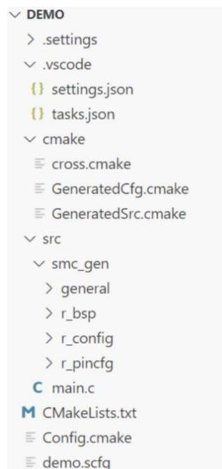
Figure 2-2 CMake CCRL project created for VS Code
