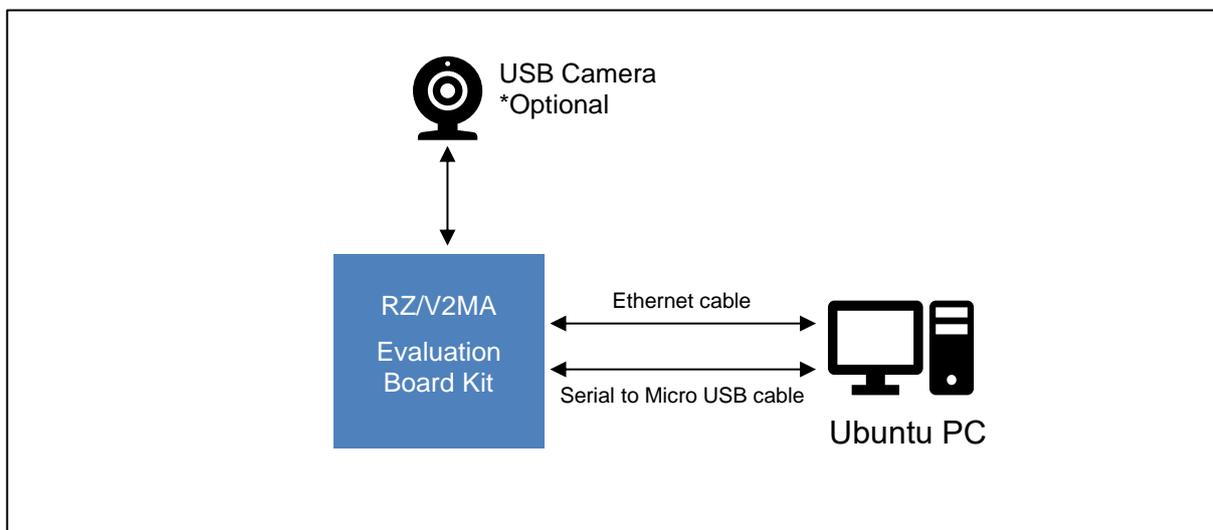
Figure 4-1 Hardware Configuration
