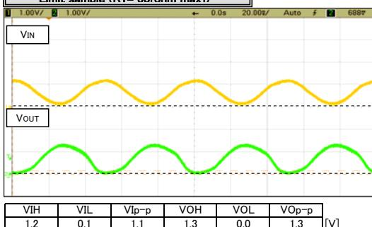
Typical sample at Vcc=5V,25deg.C    Vertical: 1V/div., Horizontal: 20ns/div.
