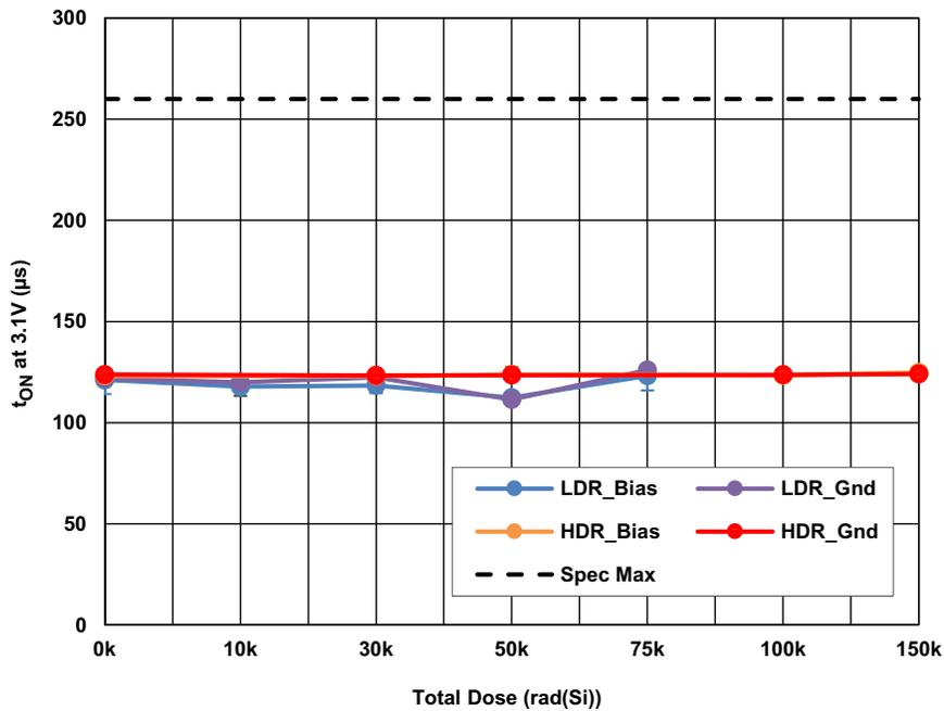
Figure 9. ISL70591SEH turn-on time at 3.1V ( $t_{ON}$ ), as a function of total dose irradiation at LDR and at HDR for biased and grounded configurations. The error bars represent the minimum and maximum measured values. The post-irradiation SMD limit is 260 $\mu$ s maximum.
