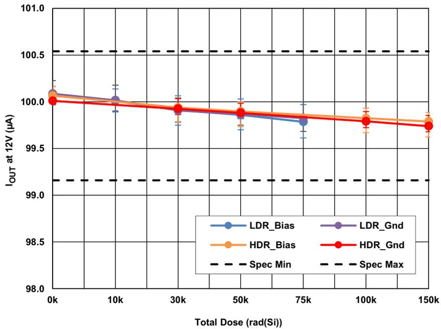
Figure 6. ISL70591SEH output current at 12V ( $I_{O12V}$ ), as a function of total dose irradiation at LDR and at HDR for biased and grounded configurations. The error bars represent the minimum and maximum measured values. The post-irradiation SMD limits are 99.16 $\mu\text{A}$  minimum and 100.54 $\mu\text{A}$  maximum.
