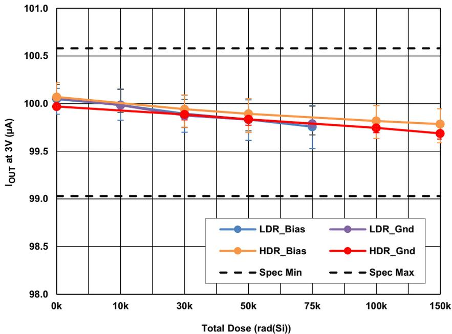
Figure 7. ISL70591SEH output current at 3V ( $I_{O3V}$ ), as a function of total dose irradiation at LDR and at HDR for biased and grounded configurations. The error bars represent the minimum and maximum measured values. The post-irradiation SMD limits are 99.03 $\mu\text{A}$  minimum and 100.58 $\mu\text{A}$  maximum.
