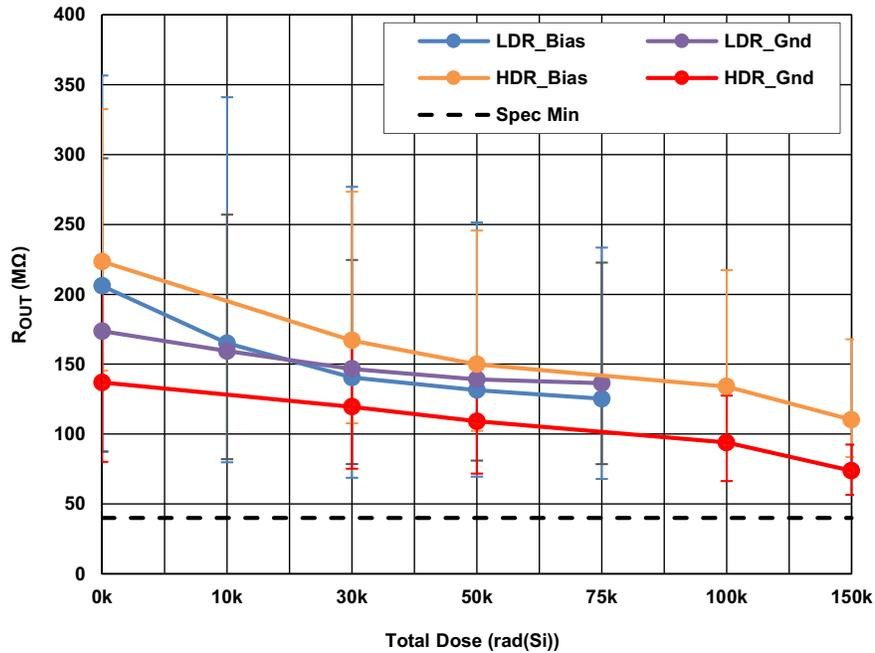
Figure 8. ISL70591SEH output impedance ( $R_{OUT}$ ), as a function of total dose irradiation at LDR and at HDR for biased and grounded configurations. The error bars represent the minimum and maximum measured values. The post-irradiation SMD limit is 40M $\Omega$  minimum.
