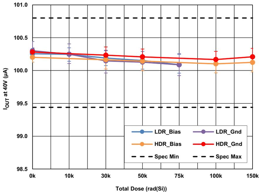
Figure 3. ISL70591SEH output current at 40V ( $I_{O40V}$ ), as a function of total dose irradiation at LDR and at HDR for biased and grounded configurations. The error bars represent the minimum and maximum measured values. The post-irradiation SMD limits are 99.44 $\mu\text{A}$  minimum and 100.80 $\mu\text{A}$  maximum.
