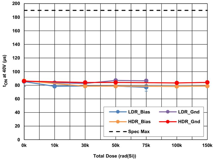
Figure 10. ISL70591SEH turn-on time at 40V ( $t_{ON}$ ), as a function of total dose irradiation at LDR and at HDR for biased and grounded configurations. The error bars represent the minimum and maximum measured values. The post-irradiation SMD limit is 190μs maximum.
