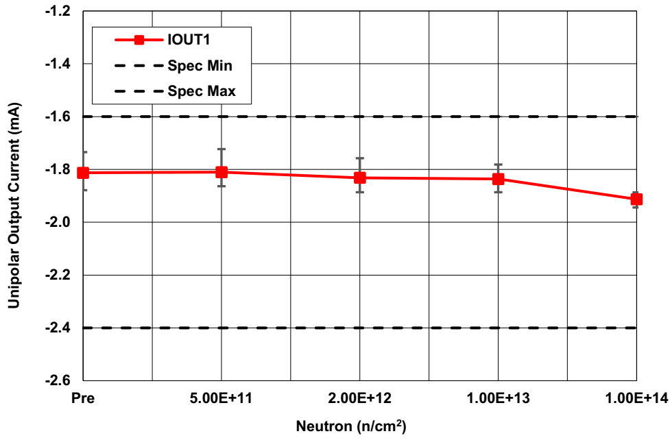
Figure 5. HS-565BxH unipolar output current ( I_{OUT1} ) with all bits on, following irradiation to each level. The error bars (if visible) represent the minimum and maximum measured values. The post-irradiation SMD limits are -2.4mA minimum and -1.6mA maximum.
