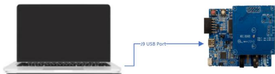
Figure 3. Connecting the VK-RA8M1 Board to the Host PC via USB Debug Port
