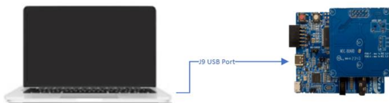
Figure 17. Connecting the VK-RA8M1 Board to the Host PC via USB Debug Port
