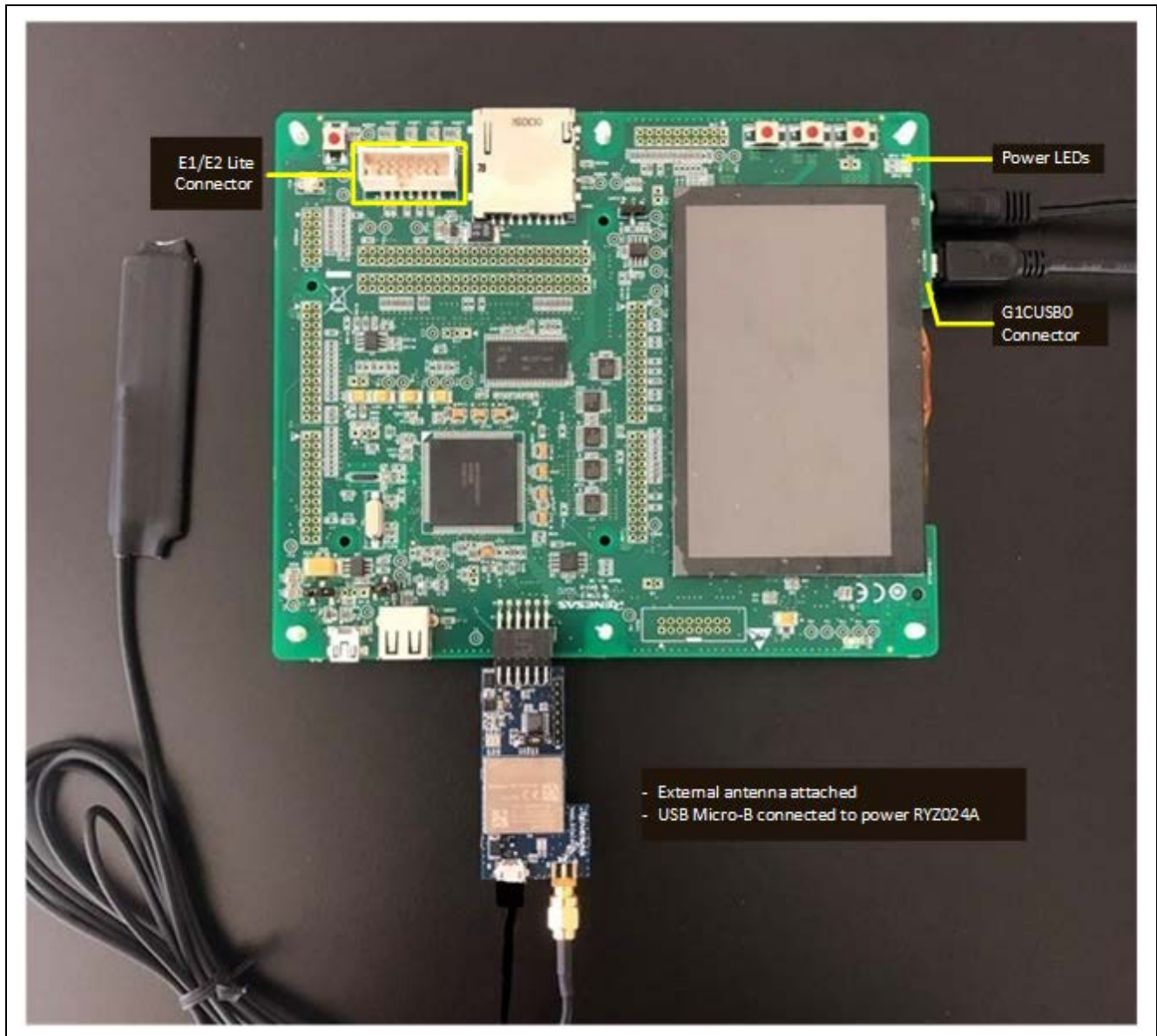
Figure 5. Connections to the RX65N-2MB Board After Flashing
