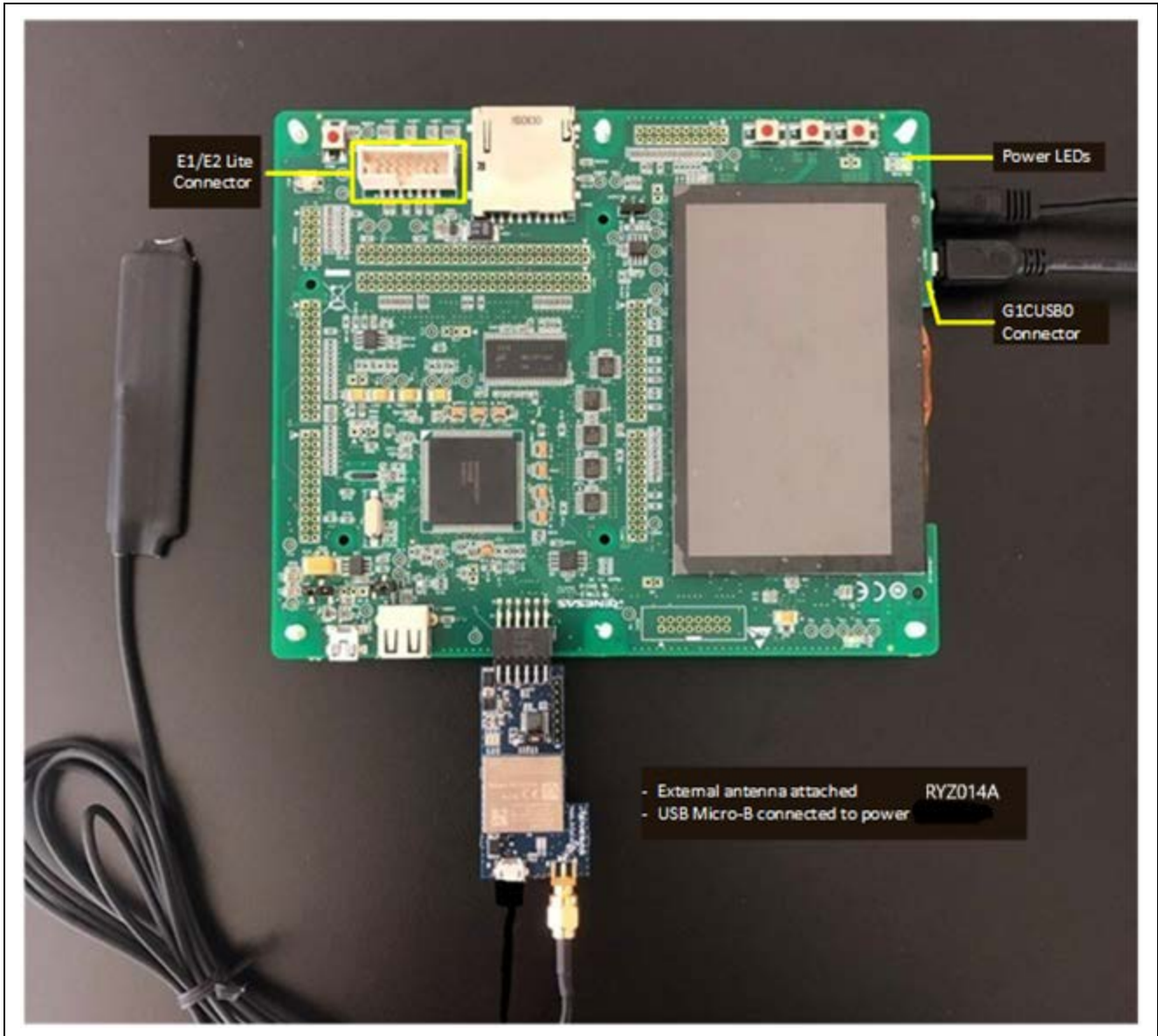
Figure 5. Connections to the RX65N-2MB Board After Flashing
