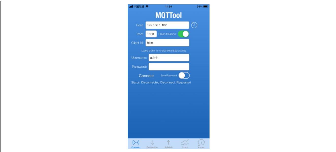
After click “Connect” button, Mosquitto receives connecting command and displays that a new connection from smartphone has been established.
