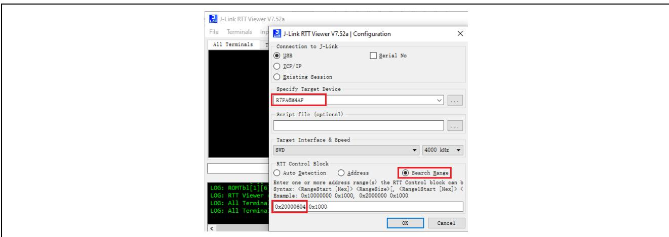
The first address of “Search Range” can be found in “\*.map” file after the demo code is built. Please open “\*.map” file and search “\_SEGGER\_RTT”, then copy the address assigned by compiler to this place.
