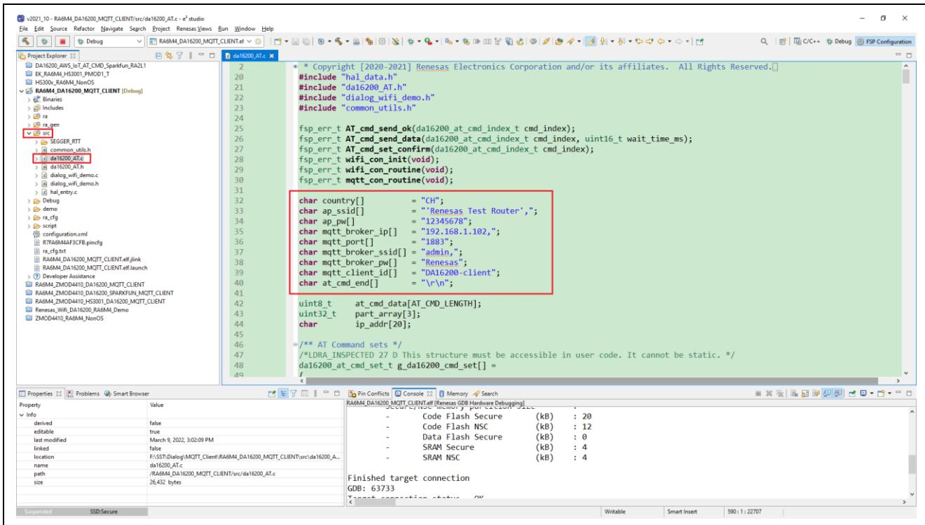
Compile the project to get the object file which can be downloaded to the chip. Then use debug function to test the sample code.
