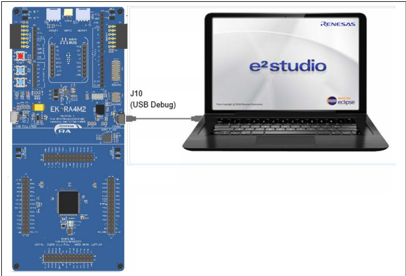
Figure 23. Connecting the EK-RA4M2 Board to the Host PC via USB Debug Port
