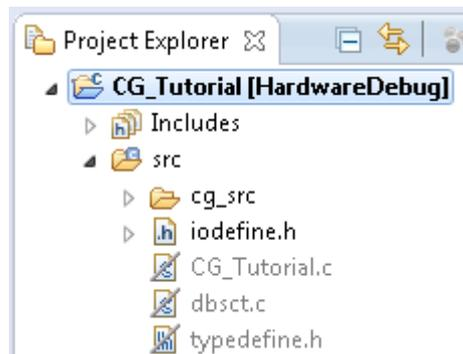
**Figure 4-21 Files excluded from the build by Code Generator**
