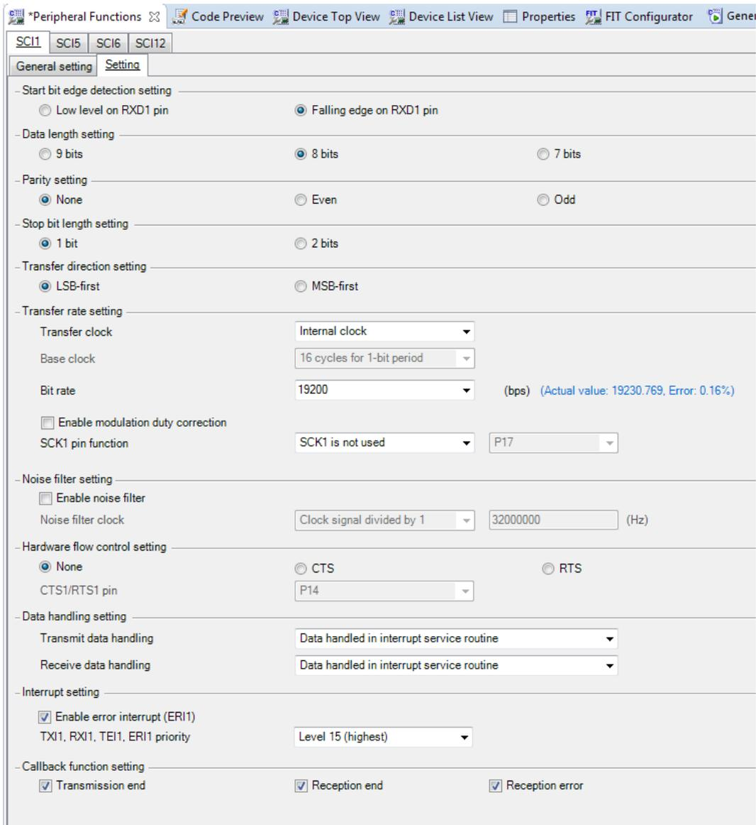
Figure 4-14 SCI1 Asynchronous Setting
