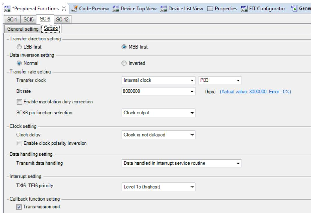
Figure 4-12 SCI6 SPI Master Setting
